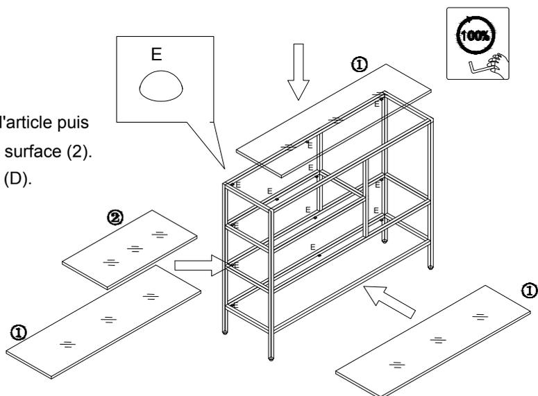
Place 24 x rubber pad (E) on the item. Install 3 x big glass (1) and 1 x small glass (2). Tighten everything completely using the Allen key (D).
